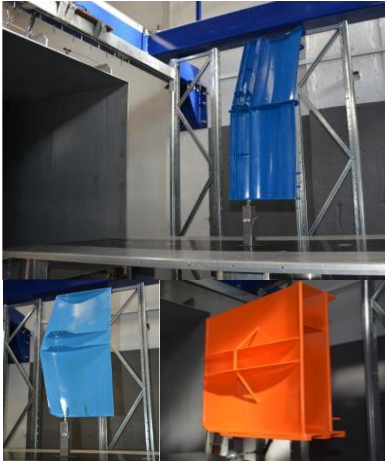
Otter boards models mounted on the six-component balance during tests (On the top, the Thyboron VF15, on the bottom the experimental models provided by our Italian manufacturers: on the left the Grilli "Fly", on the right the Mori "Biplan").
