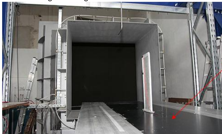
Wind tunnel: view at the open test section to the nozzle.
